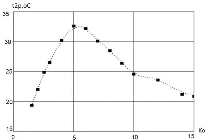
Figure 1: Dependence of the outlet temperature of the coolant at the end of the discharge process  $t_{2p}$  from the Kossovich criterion
